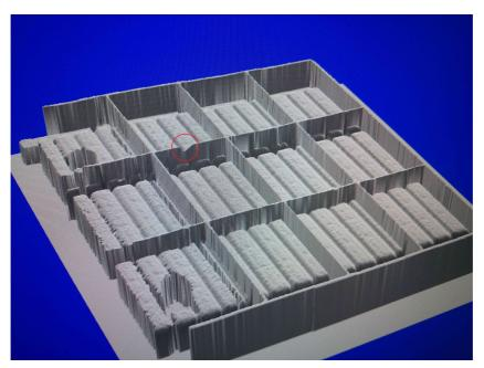
Bi-Ber's 3D scanning system employs a triangulation process that allows the safe and precise detection of broken-off chips (circled in red) in chocolate molds.
