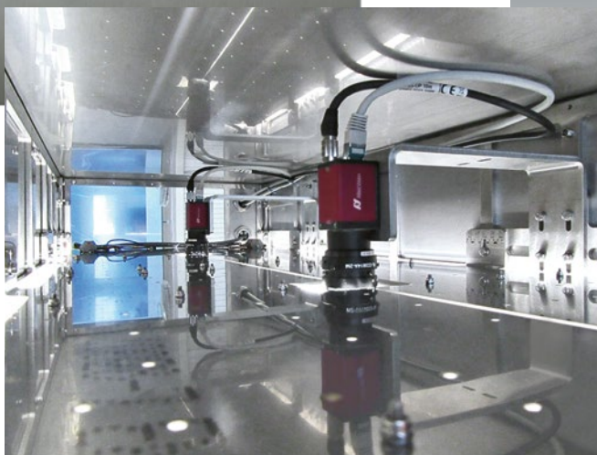
View inside the system with cameras and LED lighting
