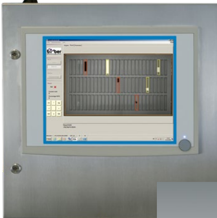
Separate control box with panel pc (with on-board image)
