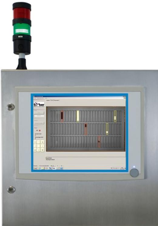
Separate control box with Panel PC (with on-board image)
